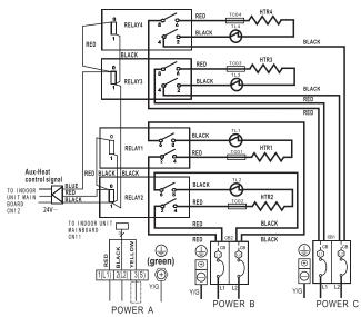
NOTE1:::::: This symbol indicates the element is optional, The wiring type of the actual unit shall prevail.
