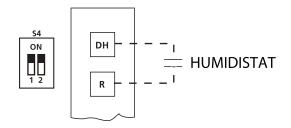
Dehumidification control requires external Humidistat at DH and R. Set S4-2 as OFF. When the humidity rises and exceeds the set value of the Humidistat, the 24V signal of DH changes to OV, the cooling system starts the dehumidification operation, and the air volume drops to 80% of the nominal cooling air volume.
