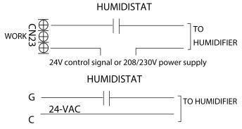
To connect a humidifier, utilize the passive signal "WORK" output (CN23) port as well as the G and C wires on the controller, and wire the humidistat and humidifier per above wiring diagram. When the fan is running, the CN23 relay will be closed, which will allow power to the humidifier when the humidistat is below humidity setpoint. If the thermostat or zone controller has an HUM interface, connect the humidifier directly to the HUM and C ports.
