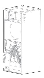
Take out the evaporator and drain pan and rotate 180° (when your equipment need to be vertical downed configuration).
